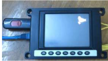
3.5" Panel PC •ARM based •2x SIO, 16x GPIO, 7 Function Keys, Audio Out •Used in applications for controlling SBCs
