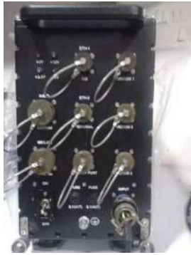
Datalink Systems ¾ ATR •3U cPCI based •Supports Data Acquisition and Control
