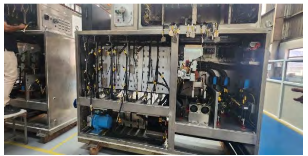
Traction Converter (under assembling process)
