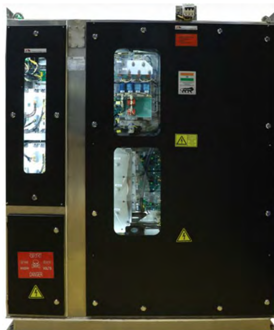
Outside view of Auxiliary converter
