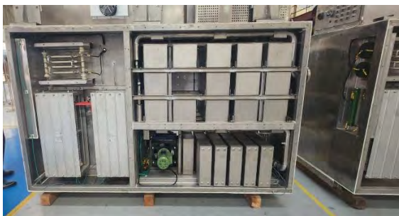
Traction Converter (under assembling process)
